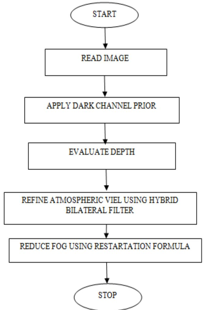
Figure 2. Flowchart of the proposed technique
